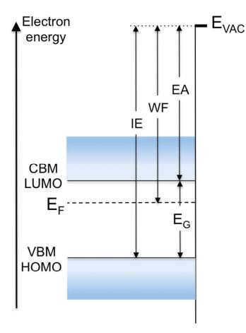
Figure 1: Energy diagram of a semiconductor with flat bands to the surface. Band edges (CBM/LUMO and VBM/HOMO), vacuum level  $E_{VAC}$ , work function WF, energy gap  $E_G$ , ionization energy IE and electron affinity EA are defined.
