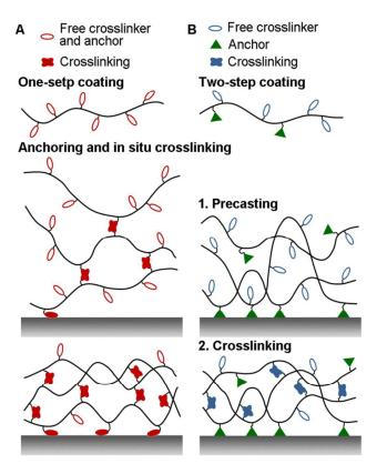
**Figure 1.** Universal coatings can be stabilized on different kinds of surfaces by interior crosslinking, which can be achieved either (A) by in situ crosslinking together with anchoring or (B) by step-wise crosslinking after formation of a precast layer.
