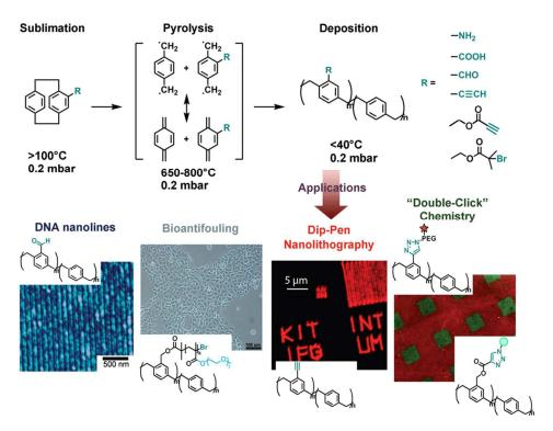
**Figure 3.** Chemical vapor deposition (CVD) polymerization with various monomers to achieve multifunctional universal coatings. Reprinted from Ref. <sup>40-43</sup> with kind permission of Wiley and The American Chemical Society.
