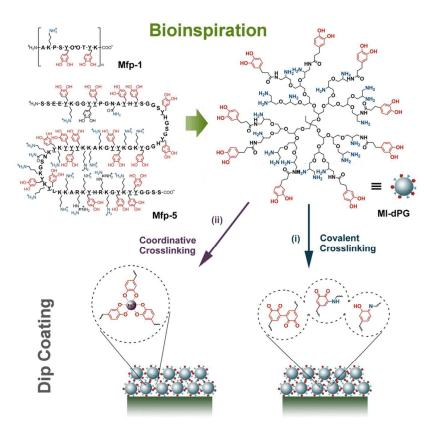
**Figure 5.** Mussel-inspired dendritic polyglycerol (MI-dPG) that mimicked the mfps by the functional groups, molecular weight, and molecular structure to result rapid covalent (postulated structure) and coordinative crosslinking for universal surface coatings. Reprinted from Ref. <sup>97</sup> with kind permission of Wiley.
