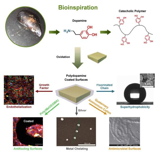
**Figure 4.** Mussel-inspired polydopamine as universal mltifunctional coatings. The structures of Mfp-1 and Mfp-5 were extracted from Ref. <sup>55</sup>. Modified from Ref. <sup>68-72</sup> with kind permission of Wiley and The American Chemical Society.
