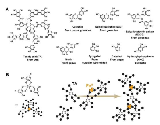
**Figure 6.** (A) Chemical structures of the natural and synthetic phenols that were identified to form universal coatings <sup>104</sup>. (B) Scheme of the assembly of iron-based coordination complexes. Reprinted from Ref. <sup>107</sup> with kind permission of AAAS.
