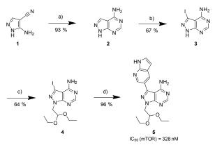
Scheme 1. Synthesis of mTOR inhibitor 5. a) Formamide, 180 °C,  $\mu$ w; b) NIS, 180 °C, DMF,  $\mu$ w; c) NaH, bromoacetaldehyde diethyl acetal, 150 °C,  $\mu$ w; d) 1*H*-pyrrolo[2,3-b]pyridine-5-boronic acid pinacol ester, K<sub>2</sub>CO<sub>3</sub>, Pd(OAc)<sub>2</sub>, PPh<sub>3</sub>, dioxane/water (10:1), 120 °C,  $\mu$ w.
