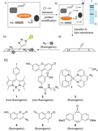
**Fig. 1** a) Schematic description of chemical blotting. i) Proteins subject to a modification reaction. (ii) The alkyne-labeled protein can be liberated from excess small molecules by SDS-PAGE iii) The alkyne-labeled protein is poised for bioorthogonal detection after it is transferred onto a blot membrane. iv) Fluorogenic, bioorthogonal reaction on the membrane surface reveal the labeled protein. b) Probes examined in this work.
