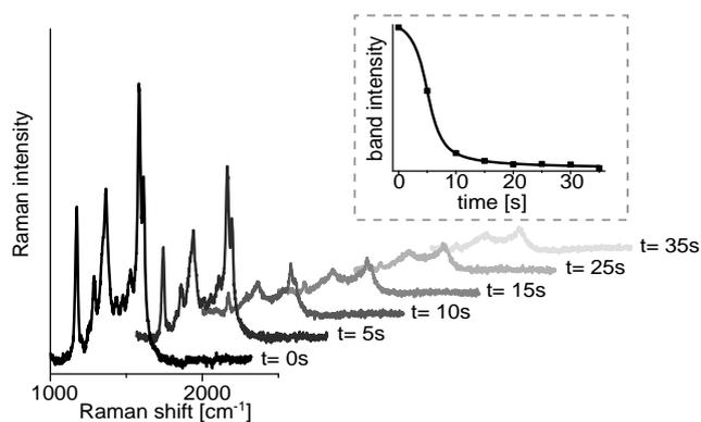
**Fig. 2** Decreasing intensity of the SERS spectra of a  $10\ \mu\text{M}$  crystal violet solution on a silver spot while potential (100 V,  $44\ \mu\text{A}$ ) and buffer flow (phosphate buffer,  $\text{pH} = 3$ ,  $22.89\ \text{mM}$ ,  $5\ \mu\text{L}\ \text{min}^{-1}$ ) is applied. The dashed box depicts the intensity of the indicator Raman band at  $1585\ \text{cm}^{-1}$ .
