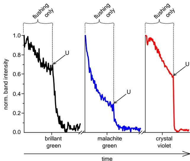
**Fig. 4** Intensity of the indicator Raman band ( $1585\text{ cm}^{-1}$ ) of three consecutively injected different dyes during the cleaning process. Only slow decrease can be observed while flushing with buffer solution, which is dramatically increased by applying high voltage. This causes substrate regeneration in only a few seconds.
