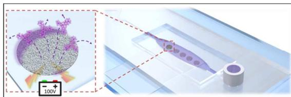
Chip-integrated electrically connected stationary SERS targets enable interference-free consecutive surface-enhanced Raman measurements by electrically assisted substrate regeneration.
