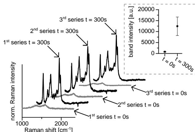
**Fig. 3** Consecutively acquired SERS spectra of clean silver substrates (grey lines) and substrates rinsed with crystal violet solution (black lines) In the dashed box the mean intensity of the crystal violet indicator band ( $1585\ \text{cm}^{-1}$ ) of fresh/cleaned and used substrates are depicted ( $n = 3$ ).
