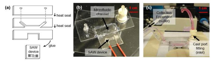
Fig. 2) (a) Schematic of SAW lysis device. (b)-(c) Images of the as-fabricated SAW device and liquid channel used to lyse exosomes.
