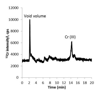
Figure 3. HPLC-ICP-MS chromatogram of Cr species in cut tobacco extracted with 2.8 mMTPABr and 4 mM EDTA (pH 8.5). 0.18mM, 1 mM EDTA as mobile phase (pH 8) at a flow rate of 0.8 mL/min.
