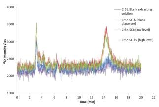
Figure 6. HPLC-ICP-MS chromatogram of Cr species in mainstream smoke from cigarette spiked two different spike levels (5.80 and 9.80  $\mu g$  g $^{-1}$  of chromium, respectively) using 2.8 mMTPABr and 4 mM EDTA (pH 8.5) as extractant. 0.18 mM, 1 mM EDTA (pH 8) as mobile phase at a flow rate of 0.8 mL/min..
