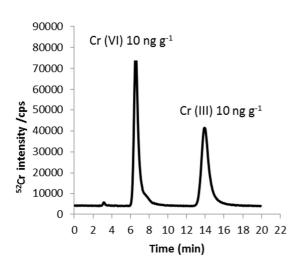
Figure 2. HPLC-ICP-MS chromatogram of Cr(VI) and Cr(III) in an aqueous standard solution (10 ng g $^{-1}$  of each Cr species). 0.18 mM tetrapropylammonium bromide (TPABr), 1 mM EDTA (pH 8) as mobile phase at a flow rate of 0.8 mL/min.
