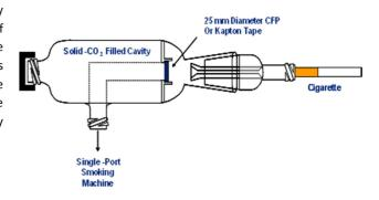
Figure 1. A schematic of the smoking glassware with a dry ice chamber. The cigarette is fitted into the glass tube on the right and a plastic tube is used to connect to a single-port smoking machine. During the experiment, the glass tube was inserted further so that the smoke from the cigarettes sticks to the CFP or a Kapton tape directly. The cap for the dry ice chamber is not kept tight during smoking in order to prevent any increase in pressure in the chamber.
