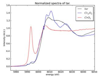
Figure 8. Normalised absorption spectra of the mainstream smoke condensate (tar) sample collected on a Kapton substrate and the two Cr standards.
