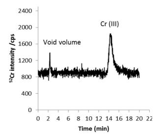
Figure 9. HPLC-ICP-MS chromatogram of Cr species in mainstream smoke spiked with 1 ng  $\rm g^{-1}$  Cr(VI) (added to the extractant). 0.18 mM, 1 mM EDTA (pH 8) as mobile phase at a flow rate of 0.8 mL/min.
