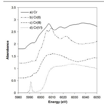
Figure 4. Normalized Cr K-edge XANES spectra of a) Cr(0) metal, b) Cr(II) Acetate, c)  $Cr_2O_3$  and d)  $CrO_3$ . These spectra have been vertically shifted for clarity.
