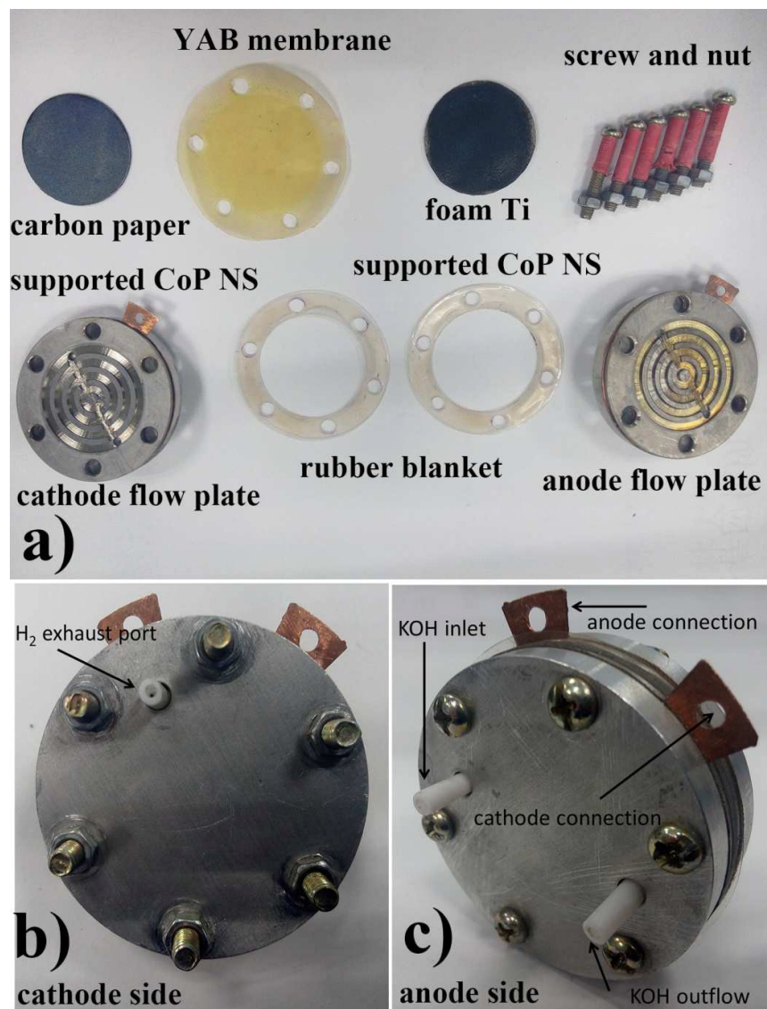
Fig. S9 Photograph of a) AEMWE cell configuration, b) cathode side and c) anode side of the electrolytic cell.
