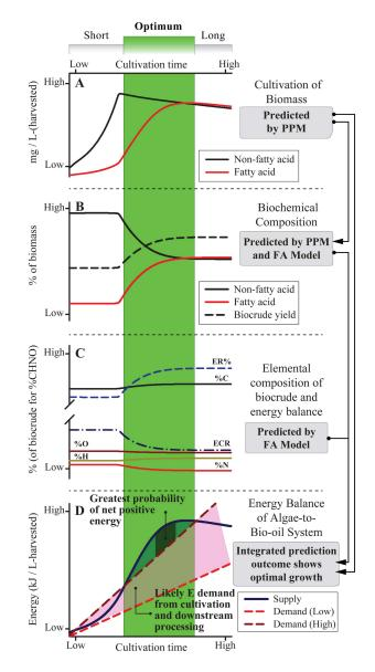
**Fig. 8** Results demonstrating the integrated modeling framework with cultivation time as the system variable. This demonstration is conceptual; quantitative analysis requires calibration of the PPM and FA models.
