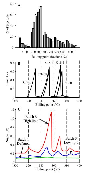
**Fig 4** A) Biocrude product boiling point (BP) distribution via SimDist analysis. Bars are ordered in increasing lipid content (Batch 1 to 8) from left to right. B) BP profile within 300–400 °C of individual fatty acids for reference to (C). C) BP profile within 300–400 °C of biocrudes derived from HTL of three representative batches of *Nannochloropsis*.
