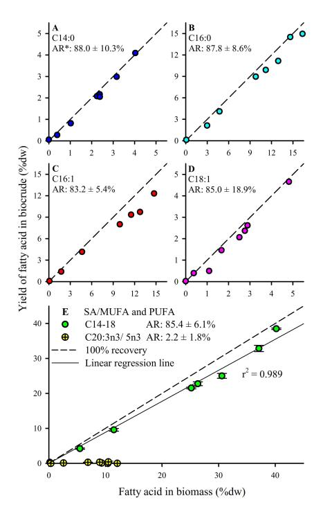
Fig. 5 Biocrude product fatty acid (FA) analysis reported as %dw yield for FAs with >1 %dw yield observed. \* Average recovery, computed using all batches except the defatted batch. Diagonal dashed line indicates 100% recovery of feedstock FA in the biocrude product. Error bars in panel E indicates min/max values from replicate analysis; error bars for individual FAs in panels A-D were smaller than the size of the symbols shown.
