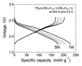
**Fig. 8.** Discharge—charge profiles over five cycles of the bulk-type all-solid-state 50 wt. %  $TiS_2/LiCB_{11}H_{12}$  |  $LiCB_{11}H_{12}$  | Li battery operated at 403 K and 0.2 C.
