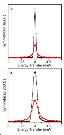
**Fig. 6.** QENS spectra at  $Q=1.35 \, \text{A}^{-1}$  showing the anion-reorientation-induced broadening in red for (a) LiCB<sub>11</sub>H<sub>12</sub> (at 433 K) and (b) NaCB<sub>11</sub>H<sub>12</sub> (at 375 K) compared to the resolution-limited elastic-scattering peaks in black observed at 200 K, below the order-disorder phase transitions. (N.B., lower instrumental resolution was used for LiCB<sub>11</sub>H<sub>12</sub>, as detailed in the Experimental Section.)
