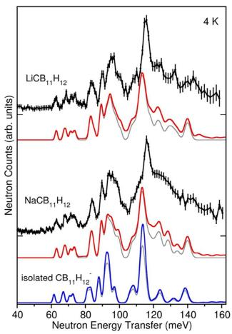
**Fig. 4.** Neutron vibrational spectra (black) of LiCB<sub>11</sub>H<sub>12</sub> and NaCB<sub>11</sub>H<sub>12</sub> at 4 K compared to the simulated one+two-phonon densities of states from first-principles phonon calculations of the optimized orthorhombic structures (red), and the isolated CB<sub>11</sub>H<sub>12</sub> anion (blue). Simulated one-phonon densities of states are depicted in grey. (N.B., 1 meV  $\approx$  8.066 cm<sup>-1</sup>.)
