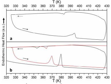
Fig. 2. Sequential heating (5 K min<sup>-1</sup>)/cooling ( $\leq$ 2 K min<sup>-1</sup>) DSC scans for (a) LiCB<sub>11</sub>H<sub>12</sub> and (b) NaCB<sub>11</sub>H<sub>12</sub> for two different cycles, the red curves measured after previously heating to 733 K. Arrows denote heating and cooling segments.
