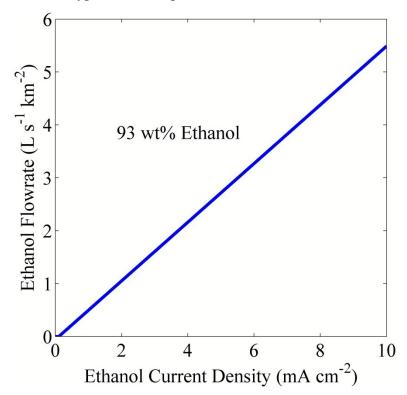
Figure 6: Flowrate of 93 wt% ethanol generated over a square kilometer area versus partial current density. Electrolyte is 13 mol%  $Cs_2CO_3$  and the crossover current density is 0.1 mA cm<sup>-2</sup>.
