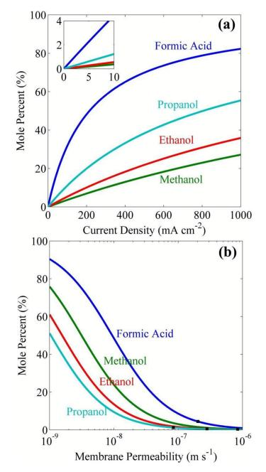
Figure 1: a) Maximum concentration of formate, methanol, ethanol, and propanol versus current density, b) Maximum concentration of formate, methanol, ethanol, and propanol versus membrane permeability. The permeabilities of these products through Nafion 117 are shown by black squares.
