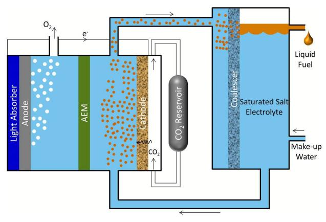
Figure 3: Schematic of advanced artificial photosynthetic system connecting a photoelectrochemical cell or PV-Electrolyzer with a liquid-liquid extractor. The liquid fuels
