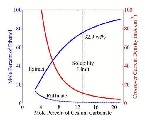
Figure 4: Equilibrium concentration of ethanol in the extract and the raffinate streams versus concentration of cesium carbonate. The crossover current density decreases with decreasing concentration of ethanol in the raffinate.
