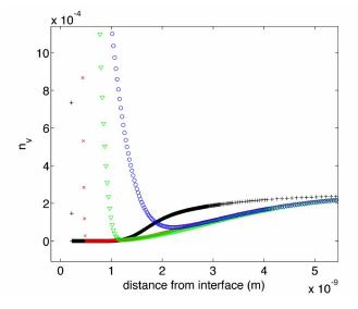
**Fig. 3** Oxygen-vacancy profiles as a function of distance from the interface at 440 °C for a (dilute) bulk dopant concentration of 0.1%. The parameters used in the simulation are those in Table 1 except for the vacancy gradient energy coefficient ( $\beta_v$ ), which is varied:  $\beta_v = 0.125 \text{ eV-nm}^2$  (+),  $\beta_v = 1.25 \text{ eV-nm}^2$  (×),  $\beta_v = 12.5 \text{ eV-nm}^2$  ( $\bigtriangledown$ ),  $\beta_v = 25.0 \text{ eV-nm}^2$  ( $\bigcirc$ )
