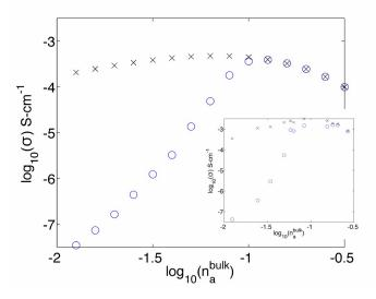
**Fig. 4** Bulk (×) and total ( $\bigcirc$ ) conductivity for gadolinia-doped ceria at 440 °C, generated from the Poisson–Cahn model for equilibrium defect concentrations and the Nakayama–Martin model for defect mobility in concentrated fluorite electrolytes. Parameters used in the model are those appearing in Table 1. Inset: experimental data for gadolinia-doped ceria from Tschöpe *et al.*<sup>23</sup>
