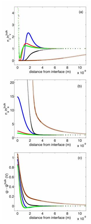
**Fig. 1** (a) Normalised vacancy concentration, (b) normalised dopant concentration and (c) electrostatic potential as a function of distance from the GB interface at 440 °C for bulk dopant concentrations of 0.01% ( $\Box$ ), 0.1% (+), 1% ( $\bigcirc$ ), 10% ( $\times$ ) and 20% ( $\bigtriangledown$ ). Parameters used in the simulation appear in Table 1
