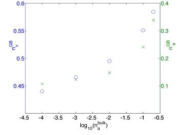
**Fig. 2** Oxygen-vacancy (), left axis) and dopant-cation (×, right axis) site fractions at the interface for 440 °C according to the Poisson–Cahn simulations, using parameters appearing in Table 1
