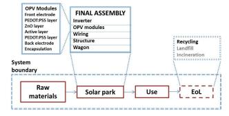
**Fig. 2.** Life cycle of the solar park including the analysed system boundaries. Materials and energy recoveries from the end-of-life stage are included in the system boundaries. Details on the system boundaries are provided in ESI-Methods† and Section 2.3.
