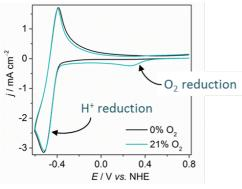
**Figure 3.** Cyclic voltammograms on a Pt disk electrode in phosphate buffer (pH 7, 0.1 M) under aerobic and anaerobic conditions at a scan rate of 50 mV s<sup>-1</sup> at room temperature.<sup>21</sup>
