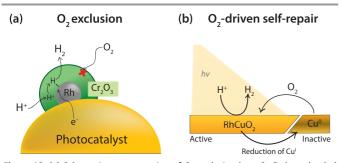
**Figure 10.** (a) Schematic representation of O<sub>2</sub> exclusion by a Cr<sub>2</sub>O<sub>3</sub> layer loaded on a Rh cocatalyst for photocatalytic water splitting.<sup>110</sup> (b) Illustration of O<sub>2</sub>-driven self-repair after photocorrosion of a CuRhO<sub>2</sub> electrode to form inactive Cu<sup>0.111</sup>
