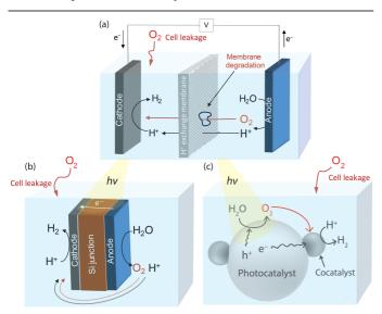
**Figure 1.** Potential routes through which a proton reducing catalyst could be exposed to  $O_2$  in (a) a standard electrolysis/PEC cell, (b) an artificial leaf and (c) photocatalytic water-splitting particles.
