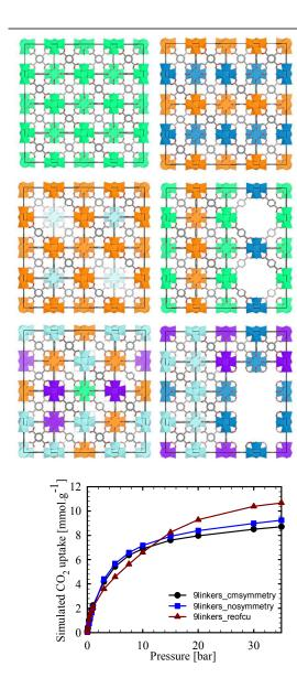
**Figure 4** (Top) Defect scenarios where all structures have the same average number of linkers per cluster (z=9) and varying heterogeneity. Each cluster is colored according to its coordination number: 12 - light blue, 11 - purple, 10 - dark blue, 9 - green and 8 - orange. (Bottom) Simulated  $\text{CO}_2$  uptake in three generalised scenarios: with symmetry, with lower symmetry and a combination of perfect *fcu* and defective *reo*.
