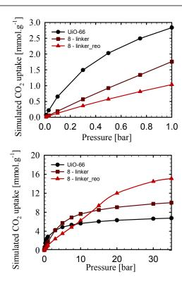
**Figure 3** Simulated CO<sub>2</sub> uptake at high pressures within a *reo* type defective structure, a structure with 8 linkers per cluster on average and a perfect *fcu* structure.
