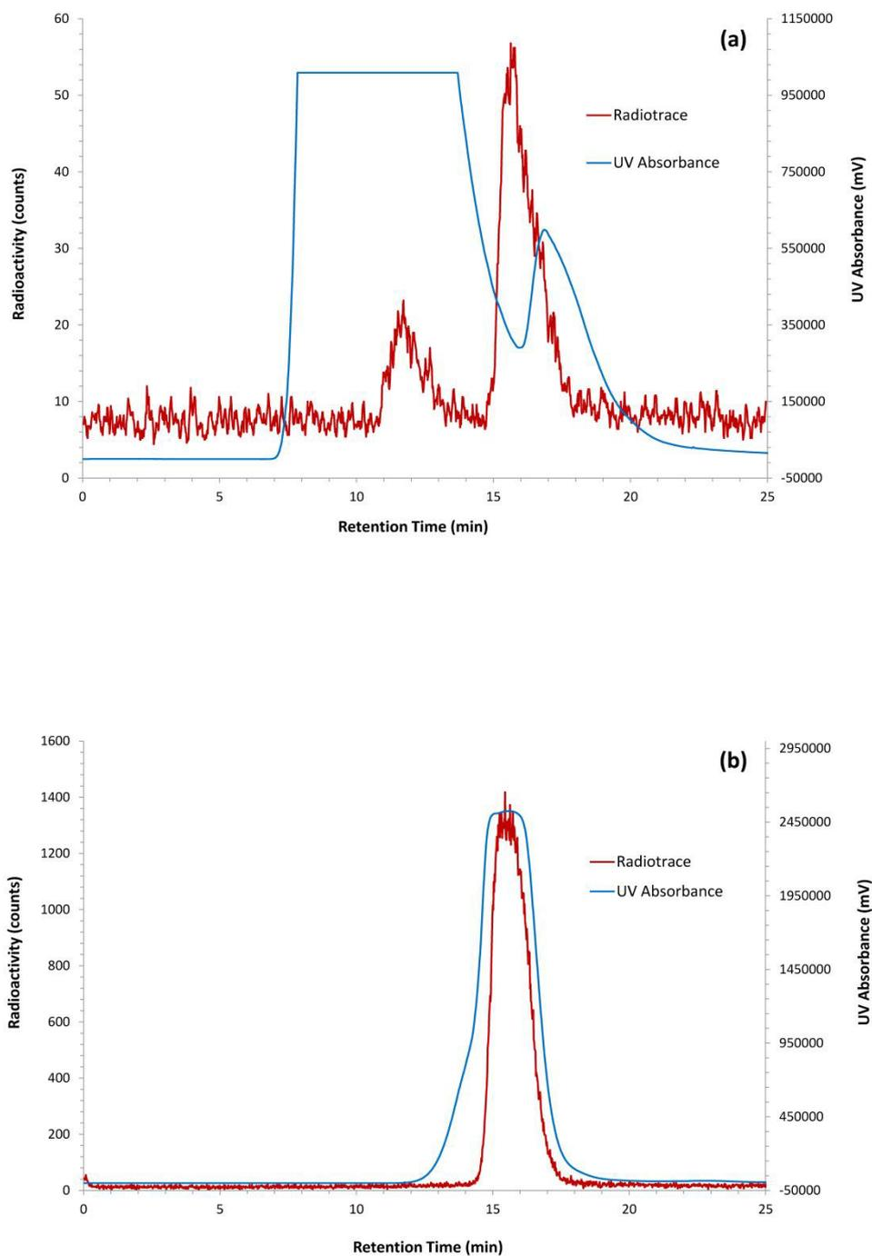
**Fig. 3** (a) SE-HPLC chromatogram obtained for  $[[^{52g}\text{Mn}]\text{Mn}(\text{CDTA})]^{2-}$  after 5 h incubation in HBS at 37 °C. The radiotracer corresponds to a simple moving average curve (order = 5). The U.V. signal generated by blood macromolecules was higher than the upper detection limit of the detector,  $R_t \approx 7\text{-}15$  min. (b) SE-HPLC chromatogram of  $[[^{52g}\text{Mn}]\text{Mn}(\text{CDTA})]^{2-}$  co-injected with non-radioactive Mn-CDTA.
