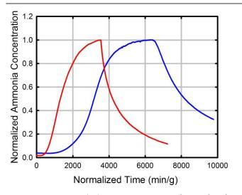
Figure 2: Downstream normalized ammonia concentration as a function of time for Cu-MOF-74 under dry (red curve) and 80 % relative humidity (blue curve).
