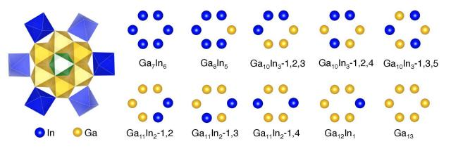
Fig. 2 Polyhedral representation of the tridecameric cluster. Assuming substitution of outer sites only, the possible isomers for the various In-substituted species are represented by the amber and blue circles, depicting In in blue and Ga in amber.
