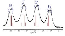
*Figure 3* Hydride resonance in <sup>1</sup>H NMR spectrum of Na[**3**–H], showing coupling to both <sup>11</sup>B ( $I = {}^{3}/_{2}$ ) and an *ortho*-CF<sub>3</sub> group {3× <sup>19</sup>F,  $I = {}^{1}/_{2}$ )
