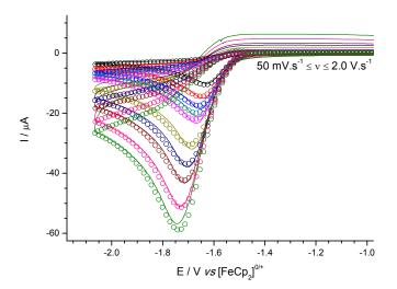
*Figure 4a* Experimental (line) and simulated (open circles) cyclic voltammograms for the reduction of **1**
