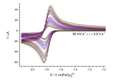
*Figure 4b* Experimental (line) and simulated (open circles) cyclic voltammograms for the reduction of **2**
