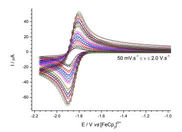
*Figure 4c* Experimental (line) and simulated (open circles) cyclic voltammograms for the reduction of **3**
