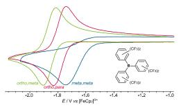
Three B{ $C_6H_3(CF_3)_2$ }<sub>3</sub> isomers have been studied as the acidic component of FLPs. *Ortho*-substituents quench H<sub>2</sub> cleavage through electron donation to the boron and steric blocking of the boron centre; as shown by electrochemical, structural and computational studies.
