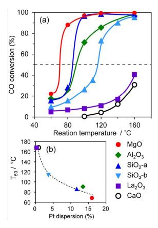
Figure 3. (a) Temperature dependence of CO conversion in PROX over various  $Pt_3Co/MO_x$  catalysts (MO<sub>x</sub> is indicated by symbols) and (b) relationship between the  $T_{50}$  and Pt dispersions.
