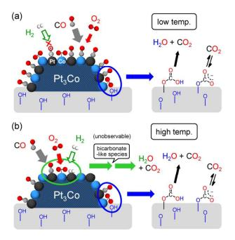
Scheme 1. Proposed reaction mechanisms of PROX over Pt<sub>3</sub>Co on an oxide support at (a) low and (b) high temperature regions.
