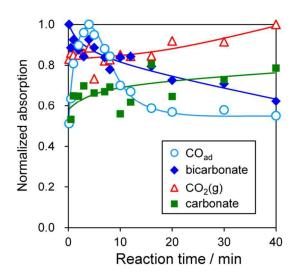
Figure 8. Changes in normalized intensities of FT-IR bands observed during high-temperature PROX (100°C).
