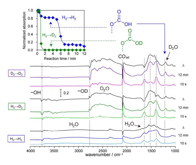
Figure 7. FT-IR spectra during low-temperature PROX over  $Pt_3Co/MgO$  with  $H_2(D_2)$  pretreatment and  $H_2(D_2)$  feeding, designated as  $H_2(D_2) \rightarrow H_2(D_2)$ . Inset shows time courses of normalized peak intensity at 1218 cm<sup>-1</sup>, corresponding to the O–H bending mode of bicarbonate.
