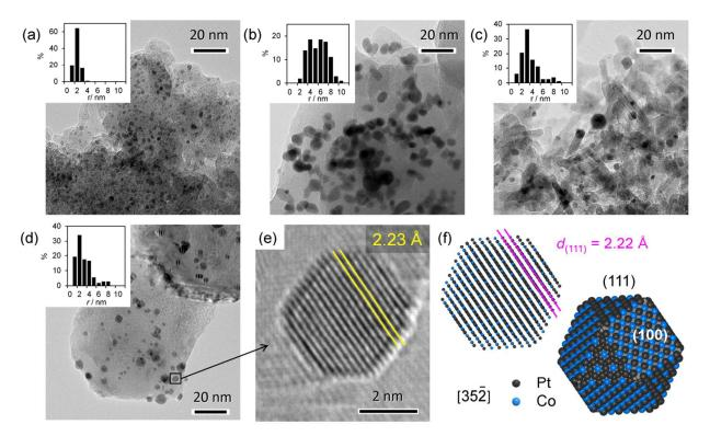
Figure 2. TEM images and size distribution of  $Pt_3Co$  nanoparticles supported on (a)  $SiO_2$ -a, (b)  $SiO_2$ -b, (c)  $Al_2O_3$ , and (d) MgO. (e) High-resolution TEM image of a single nanoparticle designated by the small square in (d). (f) Cuboctahedron models of intermetallic  $Pt_3Co$  nanocrystals projected along the [35-2] direction with small-ball (left) and space-filling (right) models.
