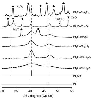
Figure 1. XRD patterns of Pt<sub>3</sub>Co catalysts.
