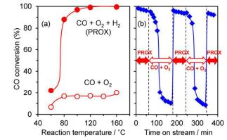
Figure 5. (a) Temperature dependence of CO conversion in PROX (CO +  $O_2$  +  $H_2$ ) and CO oxidation (CO +  $O_2$ ) over Pt<sub>3</sub>Co/MgO and (b) change in CO conversion in the presence and absence of  $H_2$  at 100°C.
