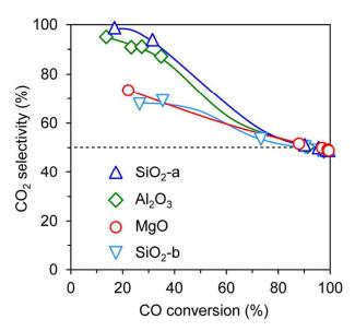
Figure 4. Conversion-selectivity curves for PROX over various Pt<sub>3</sub>Co/MO<sub>x</sub> catalysts.
