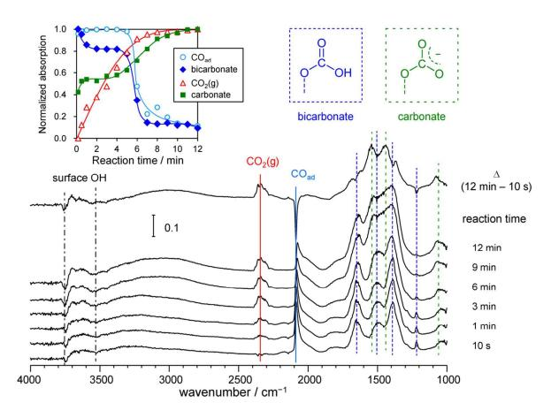
Figure 6. FT-IR spectra during low-temperature PROX over  $Pt_3Co/MgO$  (at room temperature). Inset shows the time courses of normalized peak intensity for relevant species.
