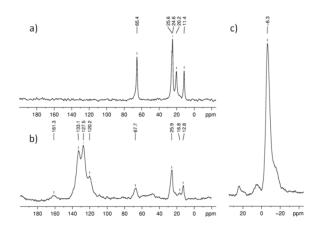
**Figure 2.** <sup>13</sup>C CP/MAS NMR spectra of **1** (a) and **2** (b) (125.7 MHz, 30 000 scans, relaxation delay of 2 s, CP contact time of 2 ms, 10 kHz spinning speed) and <sup>31</sup>P CP/MAS NMR spectrum of **2** (c) (202.4 MHz, 6 000 scans, relaxation delay of 2 s, CP contact time of 2 ms, 10 kHz spinning speed).
