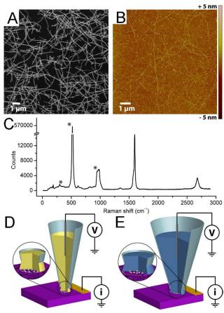
Fig. 7. E-SEM (a) and AFM (b) image of electrodeposited Pt NPs on SWCNTSa and (c) corresponding micro-Raman spectrum. Peaks marked with an \* are related to the Si/SiO2 substrate. (d) Schematic of Pt NP electrodeposition using the MCEM. (e) Schematic of the set-up used to measure ORR and MOR.Reprinted from Ref. 68, Copyright © 2014, with permission from Elsevier.
