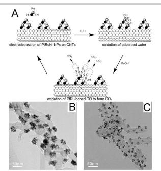
Fig. 8. A. Scheme for mechanism for PtRuNi/MWCNTs electrode surface in the methanol solution. B,C. TEM images of (B) PtRu (8:2)/MWCNTs and (C) PtRuNi (8:1:1)/MWCNTs catalysts. Adapted from Ref. 71 with permission from Elsevier, Copyright (2014).
