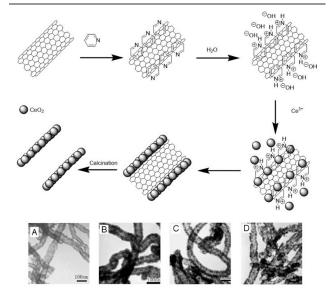
Fig. 15. Proposed mechanism for the formation of  $CeO_2$  nanotubes (top). TEM images of  $CeO_2$  nanotubes calcined for 30 min. at A) 450 °C, B) 500 °C, C) 550 °C, and D) 600 °C for 10 h. Adapted from Ref. 122 with permission from Elsevier. Copyright © 2008.
