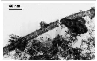
Fig. 10. TEM image of a non-homogeneous nanocomposite.<sup>100</sup> Reprinted from Ref. 100 with permission from Elsevier, Copyright (2002).
