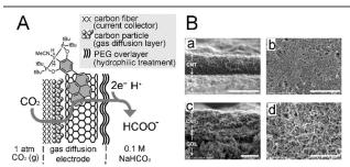
**Fig. 6.** (A) Scheme of the molecular catalyst/carbon nanotube-coated gas diffusion electrode for electrochemical reduction of CO2 to formate; (B) SEM images of the catalyst thin films on FTO (a, b) and GDL (c, d). Left (a,c): cross-section; right (b, d): top view. Adapted with permission from Ref. 48, Copyright © 2014 Wiley-VCH.
