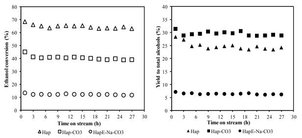
Figure 9 Ethanol conversion and total alcohols yield over stoichiometric (Hap), carbonated (Hap-CO<sub>3</sub>) and carbonate rich (HapE-Na-CO<sub>3</sub>) hydroxyapatites at 400°C and GHSV =  $5000 \text{ mL} \cdot h^{-1} g^{-1}$  as a function of time on stream.
