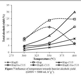
Except for Hap and HapD (represented by the dashed lines), 5 C4-C10 total alcohols yield increased while increasing the temperature up to 400°C (Figure 7). Above this temperature, the yield towards aromatics and olefins severely increased, which subsequently decreased the alcohols yield (data not shown). In Hap, the total alcohols yield remained constant at 350°C and
