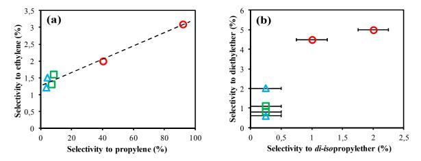
**Figure 1** (a) Selectivity to ethylene as a function of the selectivity to propylene; (b) Selectivity to diethylether as a function of the selectivity to *diiso*propylether (circles representing HapD and Hap, squares for carbonated apatites, namely Hap-CO<sub>3</sub> and HapNa-CO<sub>3</sub>, and triangles for carbonate-rich apatites, namely HapE-CO<sub>3</sub> and HapE-Na-CO<sub>3</sub>).
