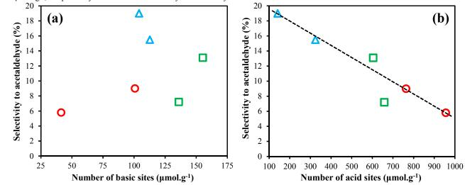
Figure 4 Selectivity of acetaldehyde as a function of (a) the number of acid sites and (b) the number of basic sites in HAPs (circles representing HapD and Hap, squares for carbonated apatites, namely Hap-CO<sub>3</sub> and HapNa-CO<sub>3</sub>, and triangles for carbonate-rich apatites, namely HapE-CO<sub>3</sub> and HapE-Na-CO<sub>3</sub>).
