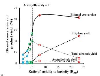
Figure 8 Ethanol conversion and major product yields at 400°C and GHSV = 5000 mL.h<sup>-1</sup>g<sup>-1</sup> as a function of the ratio of number of acid sites to the number of basic sites (red color symbols representing HapD and Hap, green color for carbonated apatites, namely Hap-CO<sub>3</sub> and HapNa <sup>65</sup> CO<sub>3</sub>, and blue color for carbonate-rich apatites, namely HapE-CO<sub>3</sub> and HapE-Na-CO<sub>3</sub>).
