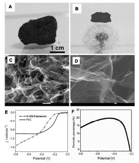
Fig. 13 (A and B) Photographs of the as-prepared superlight N-GN framework, and one with a piece of N-GN framework size of 1.8 cm x 1.1 cm x 1.2 cm standing on a dandelion. (C and D) SEM images of N-GN framework. Scale bars: (C) 10 mm, (D) 100 nm. (E) LSV curves of N-GN framework and Pt/C in O<sub>2</sub>-saturated 0.1 M KOH solution. (F) The curve of peroxide yield on the N-GN framework electrode. (Adapted with permission from Ref <sup>160</sup> Copyright 2012 Wiley-VCH Verlag GmbH & Co.)
