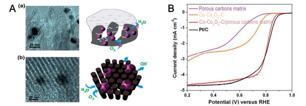
**Fig. 23** (A) The concept of the design of (a)  $Co-Co_3O_4$ -C and (b)  $Co-Co_3O_4$ -C/porous carbons matrix for promoting ORR. TEM image of  $Co-Co_3O_4$ -C/porous carbons matrix. (B) ORR polarization curves of different materials in  $O_2$ -saturated 0.1 M KOH solution at the scan rate of 10 mV s<sup>-1</sup> and the rotation rate of 1600 rpm. (Adapted with permission from Ref<sup>90</sup> Copyright 2015 Royal Chemical Society.)
