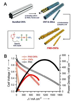
Fig. 9 (A) Synthesis of the FNS-CNTs. (B) The performance of MEAs that employ FNS-CNTs, CNTs, or Pt/C as the cathodes in alkaline fuel cells at 50 °C; open and closed circles correspond to the cell voltages and power densities, respectively. (Adapted with permission from Ref <sup>98</sup> Copyright 2014 Wiley-VCH Verlag GmbH & Co.)
