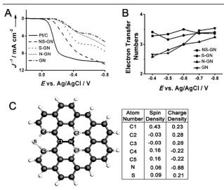
Fig. 17 (A) LSV curves of mesoporous NS-GN, mesoporous S-GN, mesoporous N-GN, mesoporous GN and Pt/C at 1600 rpm. (B) Electron-transfer numbers as a function of the overpotential of different samples. (C) Spin and charge density of GN network dual-doped by N and S. C1 has very high spin density, C2 and C3 have high positive charge density, and C4 and C5 have moderately high positive spin densities. (Adapted with permission from Ref <sup>127</sup> Copyright 2012 Wiley-VCH Verlag GmbH & Co.)
