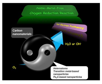
Fig. 2 Schematic illustration of the high-efficiency carbon nanomaterials-based noble-metal-free oxygen reduction electrocatalysts, which combine the advantages of carbon nanomaterials with large surface area/stable structure and heteroatoms/transition metal-based NPs/Fe<sub>3</sub>C-based NPs with high ORR electrocatalytic activity.
