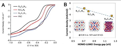
Fig. 12 (A) LSV curves of BN-GN with different compositions and Pt/C catalyst in O<sub>2</sub>-saturated 0.1 M KOH solution. (B) Experiment ORR activities vs. DFT-predicated HOMO-LUMO energy gap for BN-GN. (Adapted with permission from Ref <sup>126</sup> Copyright 2012 Wiley-VCH Verlag GmbH & Co.)
