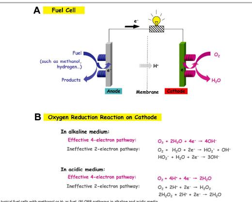
Fig. 1 (A) The typical fuel cells with methanol or H<sub>2</sub> as fuel. (B) ORR pathways in alkaline and acidic media.
