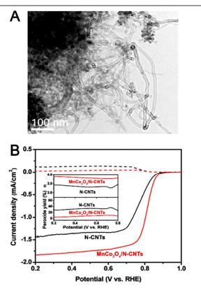
Fig. 20 (A) TEM image of MnCo2O4/N-CNTs. (B) ORR polarization curves of MnCo2O4/N-CNTs and N-CNTs. Inset: peroxide yield and electron transfer number per oxygen molecule at various potentials. (Adapted with permission from Ref <sup>81</sup> Copyright 2014 American Chemical Society.)
