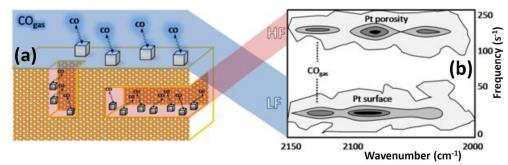
**Figure 47**. Part (a): cartoon showing CO molecules adsorbed on Pt nanoparticle located both inside the wet impregnated ZSM-5 channels and on the zeolite external surface. Part (b): 2D-PJAS-IR maps (at 573 K) of CO adsorbed on WI Pt/ZSM-5. (ion exchanged ZSM-5 at LF and colloidal impregnated at HF do not lead to any signal (HF=high frequency; LF=low frequency). Adapted from Ref.<sup>964</sup> with permission, copyright Wiley VCH, 2010.
