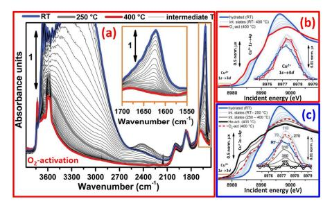
**Figure 36.** Part (a): Dehydration of the H-Cu-SSZ-13 zeolite in O<sub>2</sub> flow (30 ml min<sup>-1</sup>; O<sub>2</sub>:He = 1:1) as monitored by *in situ* FTIR spectroscopy. Spectra colors refer to different temperatures: the bold blue curve to 30 °C, bold grey
