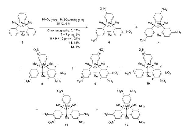
Scheme 1. Nitration of tetramethyltribenzotriquinacene 5 with standard nitration acid. The trinitro derivatives 6 and 7 and the tetranitro derivatives 8–7 were obtained as inseparable mixtures (see text).
