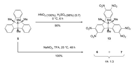
**Scheme 2.** Nitration of tetramethyltribenzotriquinacene **5** with fuming  $HNO_3/H_2SO_4$ . The trinitro derivatives **6** and **7** were obtained as inseparable mixtures (see text).<sup>[38,39]</sup>
