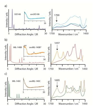
Figure 2. CuKα<sub>1</sub> powder X-ray diffraction patterns, and IR spectra, of crystalline and (inset) amorphous samples (left hand plots), complete 65 with IR spectra of the region 1450 - 1750 cm-1 (right hand plots). (a) UiO-66: dark blue,  $a_m$ UiO-66: light blue,  $a_m$ UiO-66 after 20 minutes ball milling: broken light blue, (b) MIL-140B: red, a<sub>m</sub>MIL-140B\*: orange, (c) MIL-140C: green, a<sub>m</sub>MIL-140C: brown.
