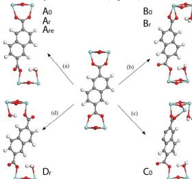
45 Figure 5. Formation of different types of defective structures upon direct binding of water on a Zr-center. The names of the defective models derived from each pathway are included for clarity. Zr - light blue, O - red, C - gray, H - white.
