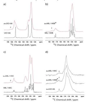
**Figure 3**. <sup>13</sup>C MAS NMR spectra of crystalline (black) and amorphous (red) samples of (a) **UiO-66**, (b) **MIL-140B** and (c) **MIL-140C**. (d) 5 Magnified view of the 150-200 ppm region of the amorphous samples. Acquisition parameter details are given in the SI.
