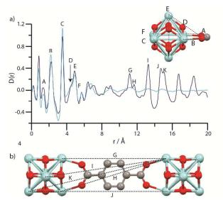
Figure 6. (a) PDF data for UiO-66 (dark blue) and  $a_m$ UiO-66 (light blue). A-F labels of peaks below 8 Å correspond to the indicated correlations in the Zr<sub>6</sub>O<sub>4</sub>(OH)<sub>4</sub> cluster (Inset). (b) Two Zr<sub>6</sub>O<sub>4</sub>(OH)<sub>4</sub> 55 units linked by a bdc ligand, and some of the significant distances corresponding to the longer r features (G-K) in (a). Zr – light blue, O – red, C – gray, H – omitted.
