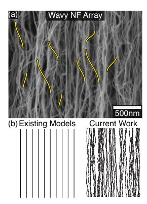
**Fig. 1** Real wavy nanofibers (NFs) and theoretical frameworks. (a) Representative high resolution scanning electron microscopy image of wavy arrays of NFs, specifically carbon nanotubes. (b) Illustration of the NF morphology normally assumed in existing theoretical frameworks, which neglect the NF waviness, and the wavy NFs with realistic stochastic morphologies generated using the simulation framework presented here.
