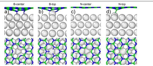
Figure 2 Atomic configurations of (0001) Mg/BNNT interface with boron (a, b) and nitrogen (c, d) vacancies at the center (a, c) and top (b, d) positions. Nitrogen, boron and magnesium atoms are depicted in blue, green and grey colors, respectively.
