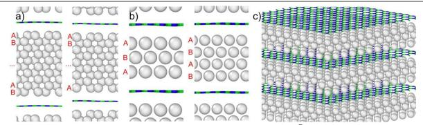
Figure 4 Atomic geometry of a composite based on individual h-BN sheets embedded between Mg matrix slabs with (a) (1010) and (b) (0001) Mg surfaces. (c) Schematic 3D view of the composite. Nitrogen, boron and magnesium atoms are depicted in blue, green and grey colors, respectively. Red letters define layer stacking.
