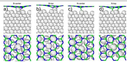
Figure 3 Atomic configurations of (1010)Mg/BNNT with boron (a, b) and nitrogen (c, d) vacancies at center (a, c) and top (b, d) positions. Nitrogen, boron and magnesium atoms are depicted in blue, green and grey colors, respectively.
