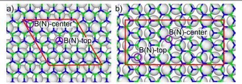
Figure 1 Atomic structure of BNNT surface located on (0001) (a) and  $(10\overline{1}0)$  (b) Mg surfaces; Simulated supercell is depicted by red frames; positions of vacancy defects created by removing B and N atoms at top and center positions are denoted by purple circles. Nitrogen, boron and magnesium atoms are depicted in blue, green and grey colors, respectively.
