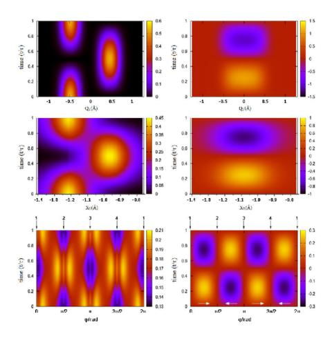
FIGURE 13: Time evolution of probability densities (left) and fluxes (right) of nuclei (top), core electrons (middle) and valence electrons (bottom) during tunnelling isomerization of  $B_4$ . Horizontal arrows in bottom right panel indicate fluxes of valence electrons, which alternate in direction in the four quadrants. Vertical arrows (bottom) labeled 1, 2, 3, and 4 indicate angular positions of nuclei B1, B2, B3, and B4 (cyclic).
