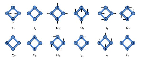
Fig. 11: Nine symmetry-adapted coordinates  $Q_1, \ldots, Q_9$  for internal nuclear motions of B<sub>4</sub>, together with coordinates  $S_x$ ,  $S_y$ ,  $S_z$  for nuclear center of mass of B<sub>4</sub>. Arrows indicate direction of motion of individual nuclei; + and - signs indicate motion either out of, or into, plane of page, respectively.
