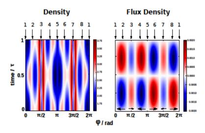
Fig. 20: Contour plots of time evolution of angular electronic probability densities (left) and flux densities (right) during Cope rearrangement of SBV in tunnelling domain. Vertical and horizontal arrows correspond to those shown in Fig. 19.
