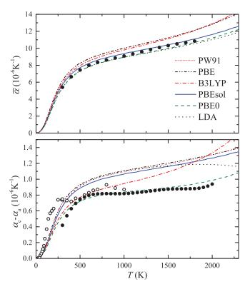
**Fig. 5** (color online) Mean *isotropic* ( $\overline{\alpha} = \alpha_V/3$ ) and *anisotropic* ( $\alpha_c - \alpha_a$ ) thermal expansion coefficient of  $\alpha$ -Al<sub>2</sub>O<sub>3</sub> calculated as a function of temperature with various DFT functionals. Full circles represent experimental data by Anderson *et al.*<sup>62</sup> for  $\alpha_V/3$  and by Munro<sup>72</sup> for  $\alpha_c - \alpha_a$ ; empty circles are data from White and Roberts.<sup>73</sup>
