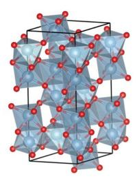
**Fig. 1** (color online) Graphical representation of the atomic structure of corundum ( $\alpha$ -Al<sub>2</sub>O<sub>3</sub>, space group  $R\overline{3}c$ ): aluminum is colored in gray, oxygen in red. AlO<sub>6</sub> octahedra and lattice parameters of the conventional cell are also represented.
