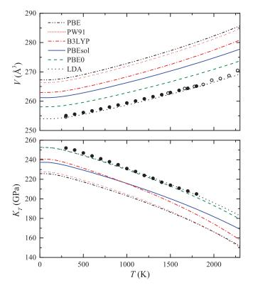
**Fig. 4** (color online) Dependence of the conventional cell volume, *V*, and bulk modulus, *K*, of  $\alpha$ -Al<sub>2</sub>O<sub>3</sub> on temperature, as computed with different DFT functionals at the quasi-harmonic level. Full and empty circles correspond to experimental data by Anderson *et al.*<sup>62</sup> and Fiquet *et al.*,<sup>63</sup> respectively.
