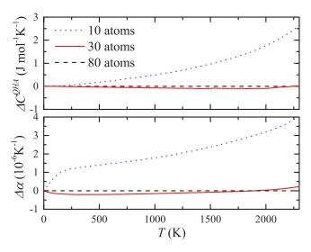
**Fig. 3** (color online) Convergence of thermal expansion coefficient  $\alpha_V(T)$  and  $C^{QHA}$  (see equation 4) of  $\alpha$ -Al<sub>2</sub>O<sub>3</sub> as a function of the adopted SC size. Differences,  $\Delta \alpha$  and  $\Delta C^{QHA}$ , are reported with respect to the SC containing 80 atoms. All results are obtained with the PBE0 functional.
