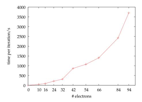
FIG. 4. Averaged CPU times for one iteration of one excitation vector in seconds, reveling a quadratic scaling of the MRA method as implemented. The molecules employed are water (10 electrons), formaldehyde (16 electrons), cyclopropane (24 electrons), acetone (32 electrons), benzene (42 electrons), norbornane (54 electrons), thymine (66 electrons), camphor (84 electrons) and phenantrene (94 electrons).
