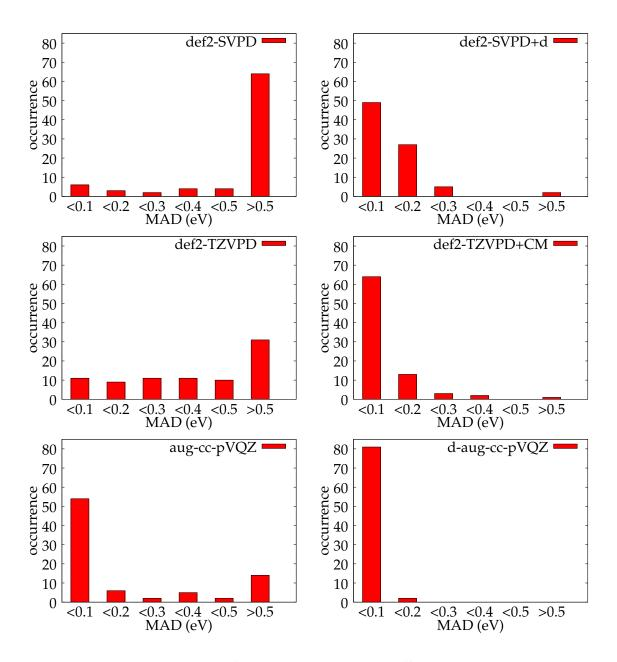
FIG. 2. Graphical representation of errors obtained using different basis sets compared to the MRA limit. Included are singlet and triplet states of the test set of 7 molecules. The total number of states is 84. Conventional basis sets are not able to account for Rydberg states and additional diffuse functions have to be used. MRA, on the other hand, is able to achieve accurate results for all states without special considerations.
