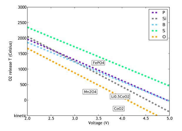
Figure 4 Linear-least squares fits to the data presented in Figure 3, separated by polyanion. Several well-known cathode materials are indicated on the plot in semitransparent text boxes.
