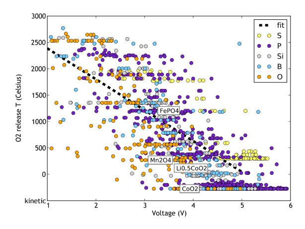
Figure 3 Computed voltage versus computed decomposition temperature for 1409 cathodes investigated by high-throughput computation. At very low temperatures, we
