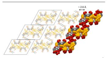
Figure 3: Bilayer arrangement for complex **1** in the absence of  $(MIPM)_2Bz^{2+}$  cations showing bilayer segments comprised of four calixarene anions and four phosphonium cations.
