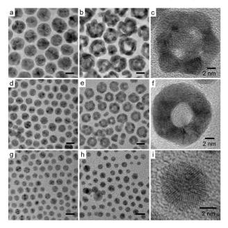
Fig. 4. (a) 15 nm (d) 8 nm (g) 6 nm MT Ag NPs and (b, e, h) after galvanic replacement with dropwise addition of 1 ml 0.2 mM AuCl<sub>3</sub> solution. HRTEM of AgAu (e) nanocage, (f) nanoring and (i) solid alloy NP.
