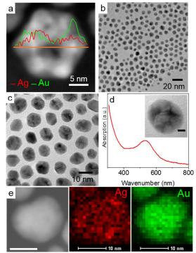
**Fig. 6.** (a) STEM image and EDX line scan of 15 nm MTP after galvanic replacement. (b) Galvanic replacement of 9 nm MTP at 100 °C with rapid addition of 1 ml of 0.2 mM AuCl<sub>3</sub>. (c) AgAu alloy NPs after rapid addition of 2 ml of 0.2 mM AuCl<sub>3</sub> solution to 6 nm NPs. (d) UV-vis spectrum of NPs in c. Inset shows HRTEM of NPs in c. Scale bar = 2 nm. (e) Elemental EDX mapping alloy NPs shown in c.
