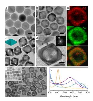
**Fig. 1** TEM image of (a) single crystal Ag NPs. After dropwise addition of (b) 0.25 ml and (c) 1 ml of AuCl<sub>3</sub>. Scale bar a-c is 10 nm. (d) HRTEM of hollow octahedral NP. (e) Elemental EDX mapping of octahedral NPs. (f) galvanic replacement of truncated cubic NPs. Inset: truncated cubic NPs. Scale bar is 10 nm. (g) UV-vis spectra of NPs showing red-shift in LSPR.
