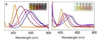
Fig. 5. UV-vis spectra of (a) 14 nm MTP and (b) 6 nm MTPs after dropwise addition of 0.2 mM  $AuCl_3$  in DCB. Inset shows photograph of NP solutions. The numbers represent each spectra from left to right. The spectrum for vial 6 is after addition of excess Au precursor is not shown.
