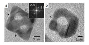
Fig. 3. Pinhole formation on {111} facet of (a) octahedral nanocage and (b) octahedral nanoring.
