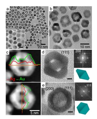
**Fig. 2.** (a-b) Galvanic replacement of 9 nm single crystal Ag NPs with addition 1.5 ml of Au solution. Inset in a shows 9 nm parent single crystal NP. Scale bar = 10 nm. (c) EDX line scan across the same NP. HRTEM of hollow AgAu alloy (d) truncated octahedral and (f)
