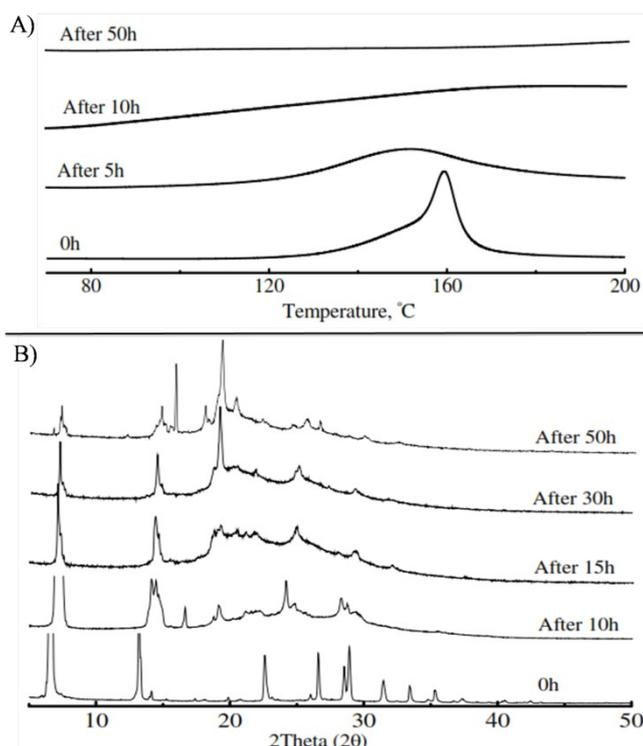
**Fig. 4** A) Overlay of DSC spectra of crystals of **1** kept at 100 °C for different durations showing the gradual decrease of exothermic peak with time. B) Overlay of P-XRD spectra of crystals of **1** kept at 100 °C for different durations showing the gradual conversion of monomer to polymer without losing crystallinity
