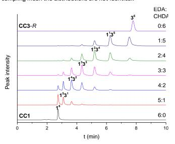
Fig. 3 Off-line HPLC analysis of cages  ${\bf CC1}$ ,  ${\bf CC3}$ , and mixtures containing all ratios of EDA to CHDA. The product distribution can be shifted by changing the diamine ratio using the flow system.
