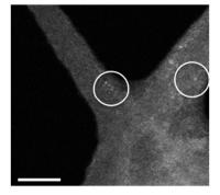
Fig. 3 TEM image of  $Cu_{16}Co_{16}$ @PAMAM-G5-Pyr. White circles highlight individual particles. Scale bar corresponds to 20 nm.
