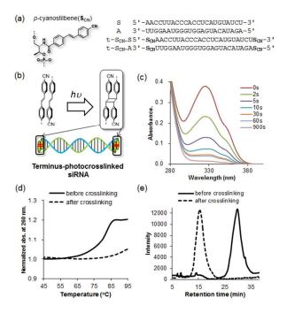
**Figure 1.** (a, b) Photo-crosslinking of *p*-cyanostilbenes in  $t-S_{CN}-S/t-S_{CN}-A$ . UV-vis spectra (c), melting curves (d), and HPLC profiles (e) of each siRNA before and after irradiation at 340 nm are shown.
