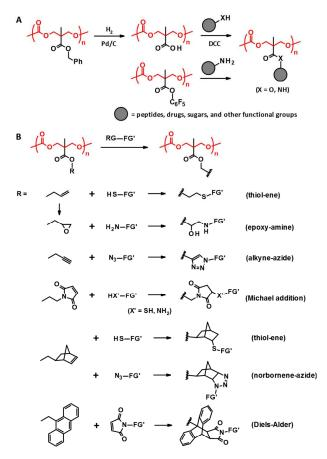
**Figure 4.** Post-functionalization of PTMC derivatives derived from bisMPA through DCC coupling and amidation (A) and "click" reactions (B). RG: reactive group, FG': functional group.
