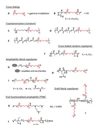
**Figure 1.** Typical examples of PTMC-based polymers applied to various biomedical applications in this review. The TMC repeating units are represented in red.
