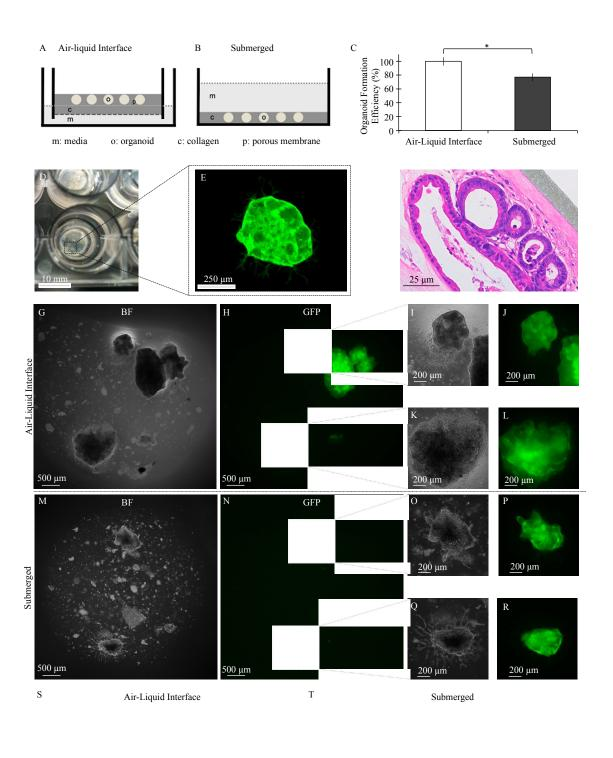
**Figure 1.** Schematic of A) air-liquid interface and B) submerged configurations used to culture primary adult murine intestinal organoids in collagen I matrices, with "c" indicating collagen I, "o" indicating organoids, "m"
