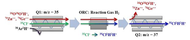
Fig. 5 Chlorine determination by ICPQQQMS in MS/MS mode with H2 as reaction gas.
