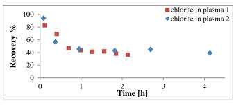
Fig. 4 Degradation of chlorite in human plasma. The time was recorded right after spiking. The recovery rates were plotted against the IC-ICPMS injection time.
