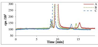
Fig. 3 IC-ICPMS gradient time optimisation, detected at m/z 35. A: 10-80 mM KOH in 0-5 min. B: 10-80 mM KOH in 0-3 min. C: 10-80 mM KOH in 0.00-0.01 min.
