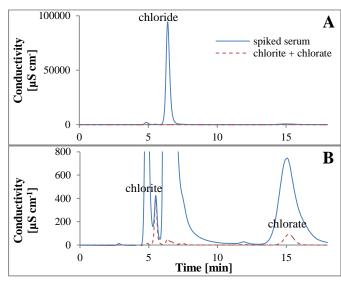
**Fig. 1:** IC chromatograms (30 mM KOH isocratic with suppressed conductivity detection) of a reference serum (1+9) spiked with 1.0 mg Cl L<sup>-1</sup> chlorite and chlorate and a standard of 1.0 mg Cl L<sup>-1</sup> chlorite and chlorate. **A:** Full-size serum chromatogram. **B:** Zoom in on the baseline.
