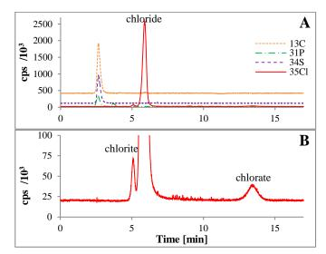
Fig. 2 IC-ICPMS chromatograms (40 mM KOH isocratic) of a sample containing serum (1+9) spiked with 5.0 mg  $L^{-1}$  chlorite and chlorate. Shown are the mass traces of carbon <sup>13</sup>C, phosphorous <sup>31</sup>P, sulfur <sup>34</sup>S (representing parts of the matrix) and chlorine <sup>35</sup>Cl. A: All chromatograms. B: Zoom in on the chlorine baseline.
