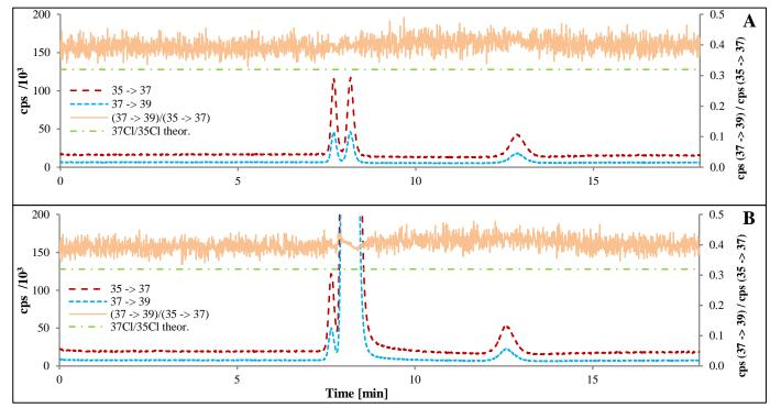
**Fig. 6** Chlorine speciation analysis by IC-ICPQQQMS. **A:** Standard solution (5.0 mg Cl  $L^{-1}$ ) **B:** Horse plasma spiked with chlorite and chlorate (5.0 mg Cl  $L^{-1}$ ). Recovery of chlorite 93 % and of chlorate 104 %.
