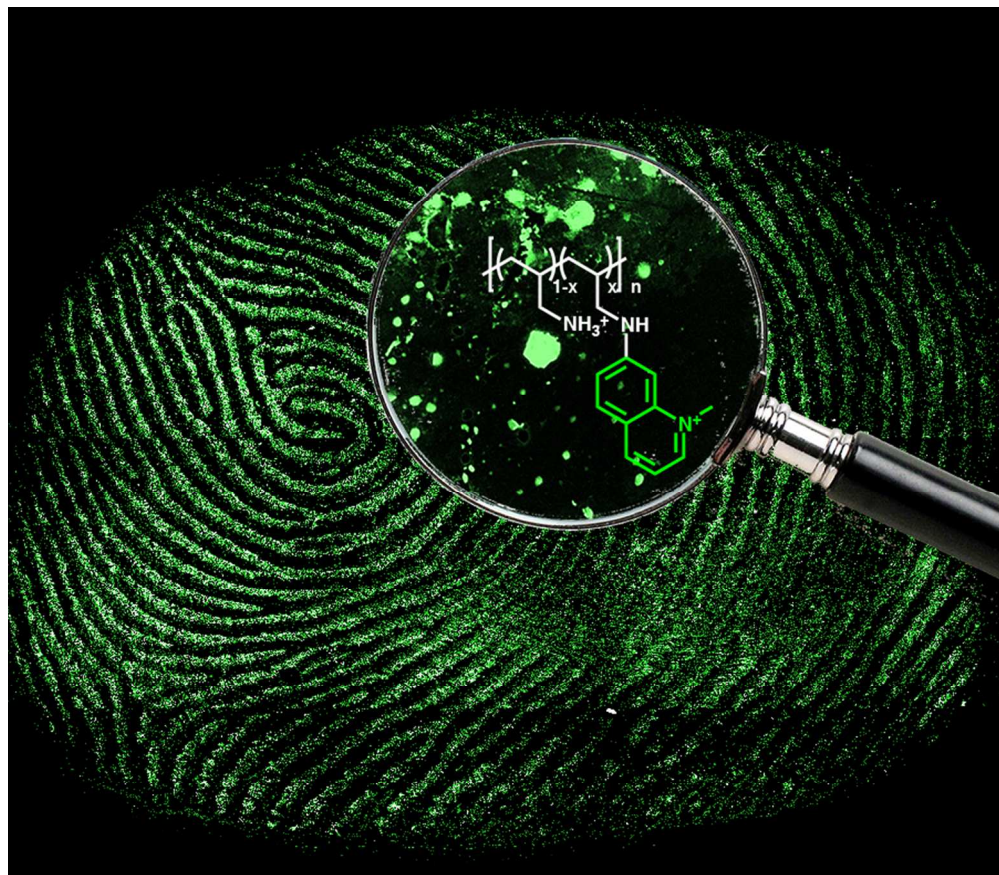
A fluorescent polyelectrolyte, poly(allylamine hydrochloride (PAH) functionalised with the 7-amino-quinolinium chromophore, has been synthesized and employed for the visualization of latent fingerprints. 319x277mm (72 x 72 DPI)
