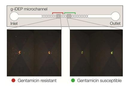
Gradient insulator-based dielectrophoresis used to generate separation and concentration of *Staphylococcus epidermis* gentamicin resistant and susceptible strains.
