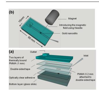
**Figure 2 (a)** top view of the funnel chip integrated with CG nanoslit film and the magnet. The needle was used to introduce the magnetic field to the detection area. **(b)** Layered structure of the microfluidic chip integrated with a CG nanoslit film.
