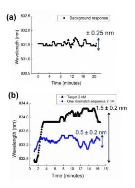
**Figure 4 (a)** The dynamic SPR response from applying the method to a blank sample (b) The dynamic SPR response from applying the method to a sample of 2 nM one mismatch sequence in comparison with the response from a sample of 2 nM perfect match sequence
