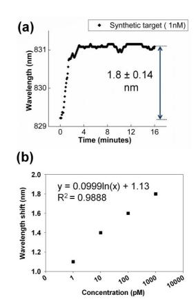
**Figure 3** (a) The dynamic SPR response that indicates the real-time progression of the hybridization of target molecule with the probe II on the CG nanoslit, (b) The calibration curve obtained for various concentration of synthetic miRNA-16-5p spiked in urine from healthy subjects
