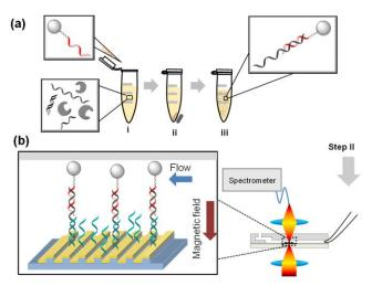
Figure 1 A schematic of the double hybridization method to detect the nucleic acid target (a) First step: isolation of the target molecule using MNPs (b) Second step: hybridizing the target molecule isolated on the MNPs with Probe II on the CG nanoslit.
