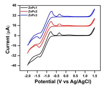
Fig. 5 Cyclic voltammogram of ZnPc1-3 in dimethylformamide.
