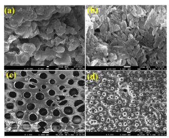
Fig. 10 Scanning electron microscope (SEM) images of ZnPc thin films prepared from chloroform: (a) ZnPc1 (b) ZnPc2 and (c) ZnPc3. (d) SEM of ZnPc3 thin films obtained from methanol.
