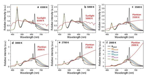
Fig. 5. The EL spectra of the six combinations of four-package R<sub>B,M</sub>A<sub>B,M</sub>B white LEDs at different CCTs with the various red phosphors and the reference ideal (Planckian) or natural (sunlight) light sources of CRI at different CCTs: (a) 6500 K, (b) 5000 K, (c) 3500 K, (d) 3000 K, (e) 2700 K, and (f) 2000 K.
