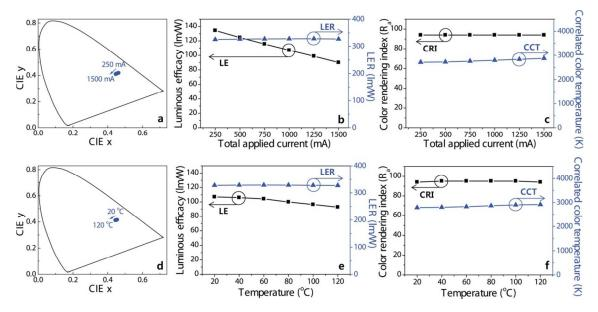
Fig. 7. Current dependence of the  $R_{N,B,M}G_{B,M}B$  white LED at 2700 K at room temperature: (a) 1931 CIE color coordinates, (b) LE and LER, and (c) CRI and CCT. The temperature dependence of the  $R_{N,B,M}G_{B,M}B$  white LED at 2700 K with a total applied current of 1000 mA: (d) 1931 CIE color coordinates, (e) LE and LER, and (f) CRI and CCT.
