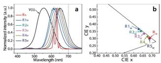
**Fig. 2.** (a) The photopic luminosity function  $(V(\lambda))$  and normalized PL spectra of six red phosphors and (b) the 1931 color coordinates of the six red phosphors.
