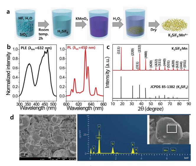
Fig. 1. (a) Schematic diagram of synthetic method of  $K_2SiF_6:Mn^{4+}$ , (b) the excitation and emission spectra, (c) powder XRD (JCPDS 85-1382 ( $K_2SiF_6$ )), and (d) FE-SEM and EDS data of the as-synthesized  $K_2SiF_6:Mn^{4+}$  phosphor.
