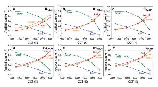
Fig. 4. The fractional applied currents of the primary LEDs in six combinations of four-package  $R_{B,M}A_{B,M}G_{B,M}B$  white LED at different CCTs with the various red phosphors: (a)  $R_{N,B,M}$ , (b)  $R1_{W,B,M}$ , (c)  $R2_{W,B,M}$ , (d)  $R3_{W,B,M}$ , (e)  $R4_{W,B,M}$ , and (f)  $R5_{W,B,M}$ .
