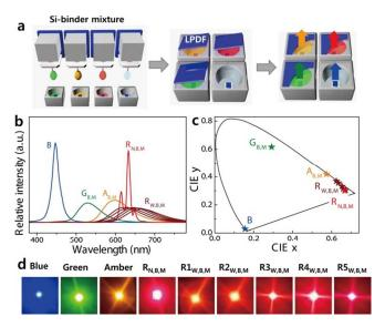
**Fig. 3.** (a) Schematic diagram of four-package white LED, (b) The EL spectra, (c) 1931 CIE color coordinates, and (d) photographs of the blue semiconductor-type LED and eight different colors of fully down-converted LPDF-capped pc-LEDs ( $G_{B,M}$ ,  $A_{B,M}$ ,  $R_{N,B,M}$ ,  $R_{W,B,M}$ ,  $R_{W,B,M}$ , and  $R_{W,B,M}$ ).
