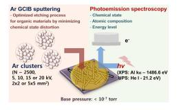
In-situ molecular distribution analysis based on photoemission spectroscopy combined with Ar Gas Cluster Ion Beam sputtering process
