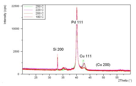
Figure 5 : XRD spectra of copper films grown on Pd films at various temperatures.
