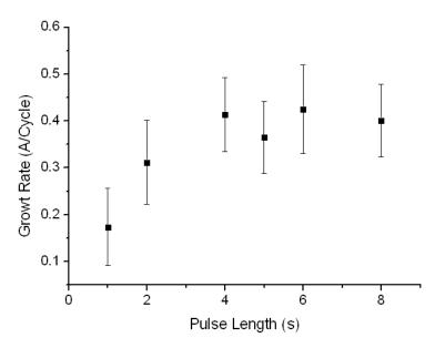
Figure 7 : Growth Rate vs precursor pulse length for Cu films grown on Pd at a substrate temperature of 220  $^{\circ}$ C; the error bars refer to the standard deviation.
