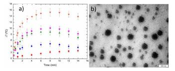
**Figure 2.** a) Temperature increments as a function of time under NIR light irradition (2.5 W cm<sup>-2</sup>, 5 min at 808 nm) for aqueous solutions of ( $\blacksquare$ ) bare PLGA NPs; ( $\blacklozenge$ ) 8  $\mu$ M free ICG, and DXSP-PLGA-ICG NPs containing ( $\bigcirc$ ) 1, ( $\blacktriangle$ ) 4 ( $\bigtriangledown$ ) and 8  $\mu$ M conjugated-ICG. b) TEM image of DXSP-PLGA-ICG NPs after irradiation (2.5
