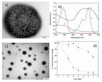
Figure 1. a) TEM image of a DXSP-PLGA NP. b) UV-Vis spectra of 1) free DOXO, 2) DXSP-PLGA NPs, 3) free ICG and 4) DXSP-PLGA-ICG NPs. c) TEM image of DXSP-PLGA-ICG NPs. d) Fluorescence stability of (■) free ICG and (●) ICG complexed to PLGA NPs. In d) lines are to guide the eye.
