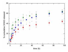
**Figure 3.** *In vitro* release kinetics of DOXO from DXSP-PLGA NPs (PLGA  $M_w = 38-54$  kDa) in aqueous serum-containing (10% FBS) medium of pH 7.4 in the absence ( $\blacksquare$ ) and presence ( $\bigcirc$ ) of irradiation (2.5 W cm<sup>-2</sup>, 5 min at 808 nm), and of pH ( $\blacktriangle$ ) 5.5 in the absence of irradiation.
